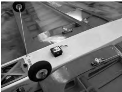
Main Sensor Module mounted on bottom of fuselage
