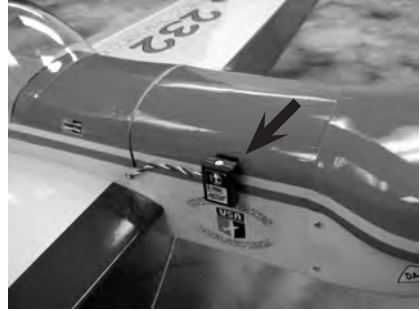
Vertical Sensor Module mounted on fuselage side
