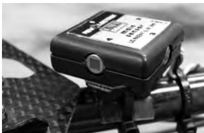
Main Sensor Module mounted on helicopter boom
