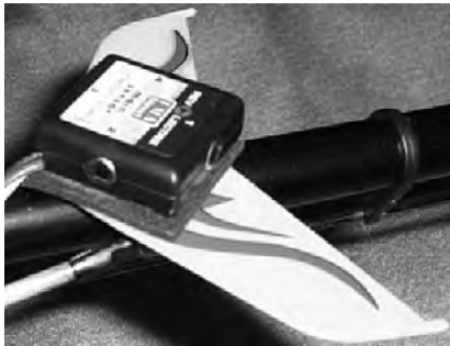
Main Sensor Module mounted on horizontal fin
