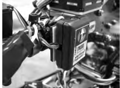
Vertical Sensor Module mounted on helicopter boom
