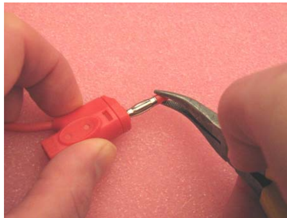
Using small pliers, remove the rubber tip from the banana plug as shown.
