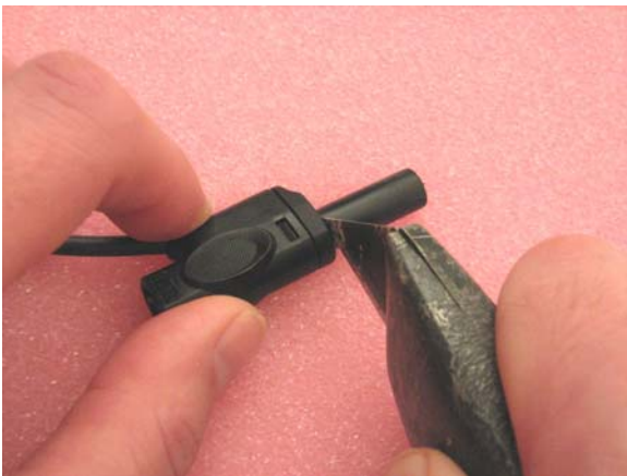
Using a utility knife, carefully cut the protective tube from around the banana plug as shown and remove.
